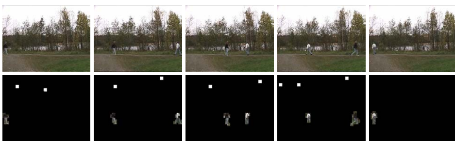
Figure 9: Frames 280, 300, 320, 350 and 380 from an outdoor test sequence where two persons are walking in front of heavily swaying trees and rippling water. There can also be some camera jitter present because of the wind.
