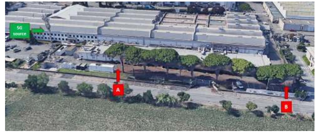
FIGURE 8. Measurement site; the measurement positions are labeled A and B; the 5G base station antenna is visible on the left.
