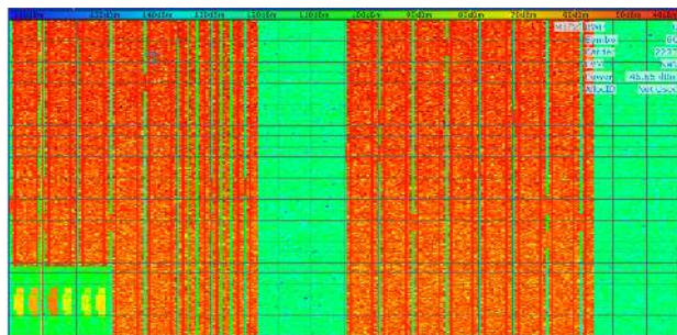
FIGURE 13. The power per RE versus the subcarriers (vertical axis) and the OFDM symbols (horizontal axis) in a frame in case of full use of the grid resources; the power level is plotted in false colors.
