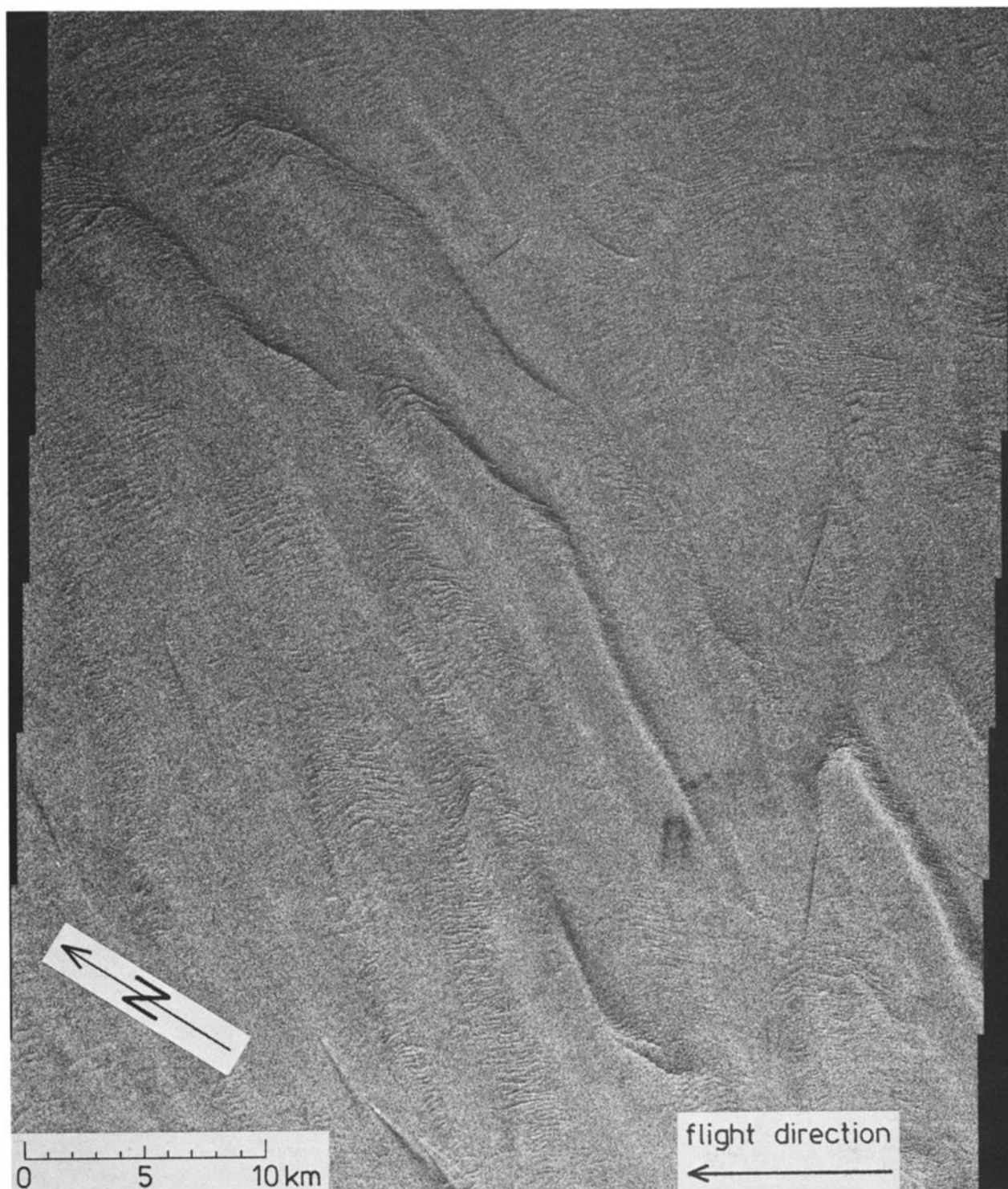
Fig. 6a. Digitally processed Seasat SAR image of the Southern Bight of the North Sea from orbit 762 (August 19, 1978, 0646 UT) with frame center at 51^{\circ}30'40''\text{N} and 2^{\circ}31'23''\text{E} . (The top part of Figure 5a is identical to the bottom part of this figure.)
