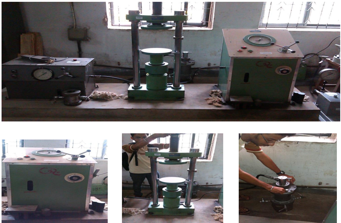
Fig. 3.10 Tri-axial test apparatus
