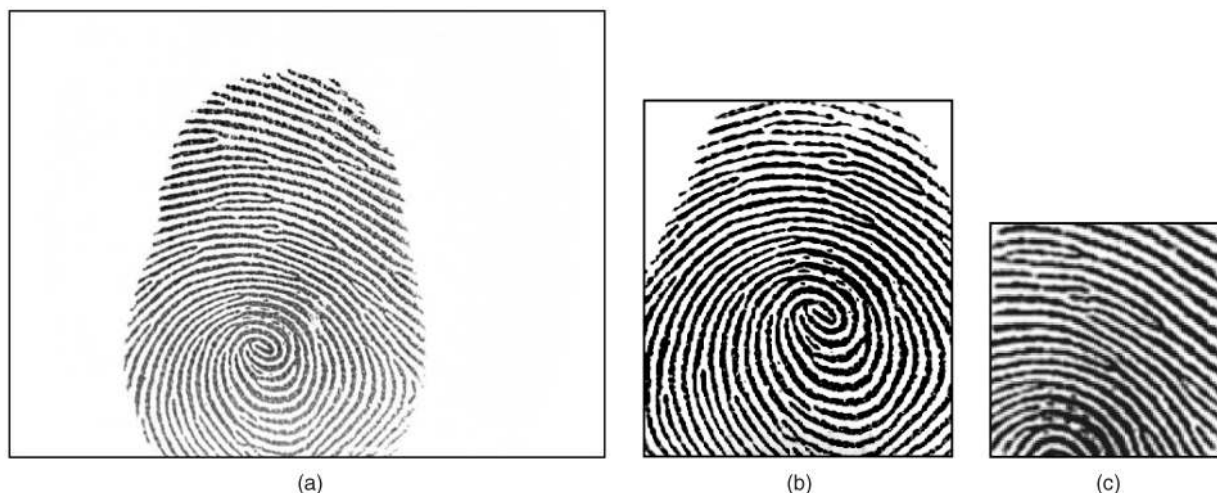
Fig. 15. Sample images from the WVU data set. Images of the same finger were acquired using three different sensors. (a) CM. (b) SG. (c) PC.
