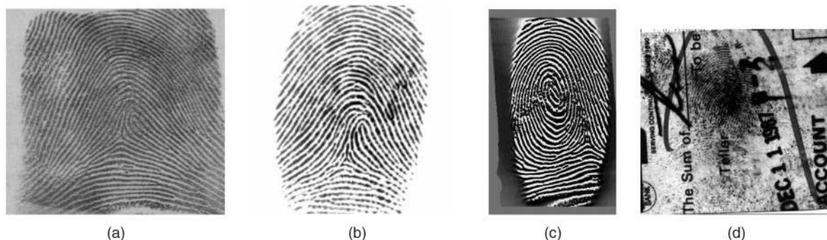
Fig. 1. Four different schemes for fingerprint acquisition. (a) Rolled print (from the NIST Special Database 4). (b) Dab print (from the FVC 2002 DB1 Database). (c) Swiped sensor print (from the FVC 2004 DB3 Database). (d) Latent print (from [3]).
