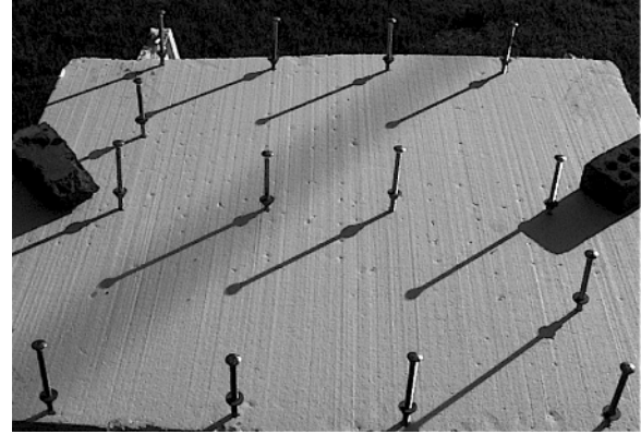
Fig. 6. Target scene of 15.24 cm tall 0.95 cm diameter carriage bolts in a block 'S' pattern.
