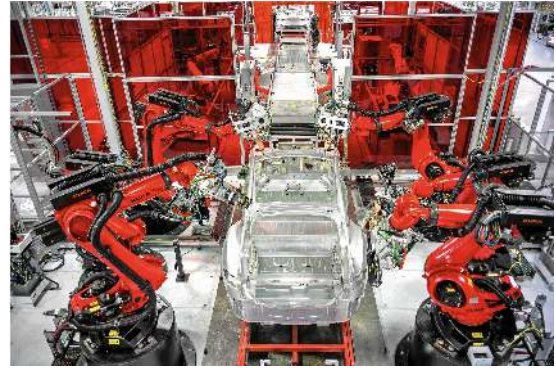
Fig. 1. Robotic assembly station in the Tesla factory. Tesla's special KUKA robots can perform different tasks [26].
