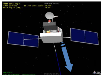
TMI reflector face illuminated before eclipse
