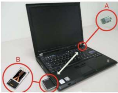
Fig. 1. Demonstration of the hardware for setting up a rogue AP. The requirement is only a laptop with two wireless adaptors: A is an internal wireless adaptor which is connected to a legitimate AP, and B is an external wireless adaptor which behaves as a legitimate AP to induce users.
