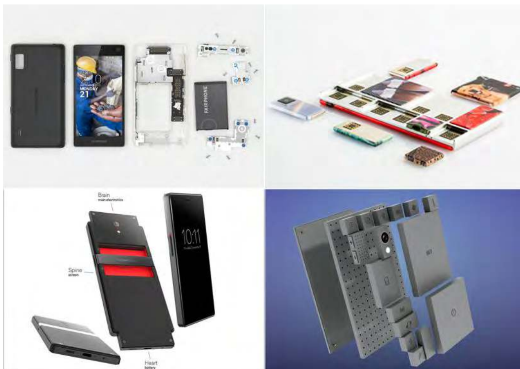
Figure 8 A range of modular smart phone concepts. Clockwise top left to bottom left – Fairphone, Google’s Project Ara, PhoneBlok and PuzzlePhone (all 2015).
