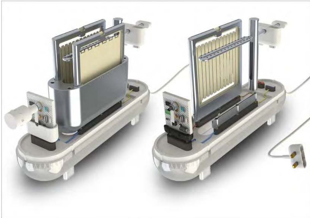
Figure 6 The prototype's design is modular with no screws, glues or hidden seals. Users would therefore be able to easily disassemble the toaster.
