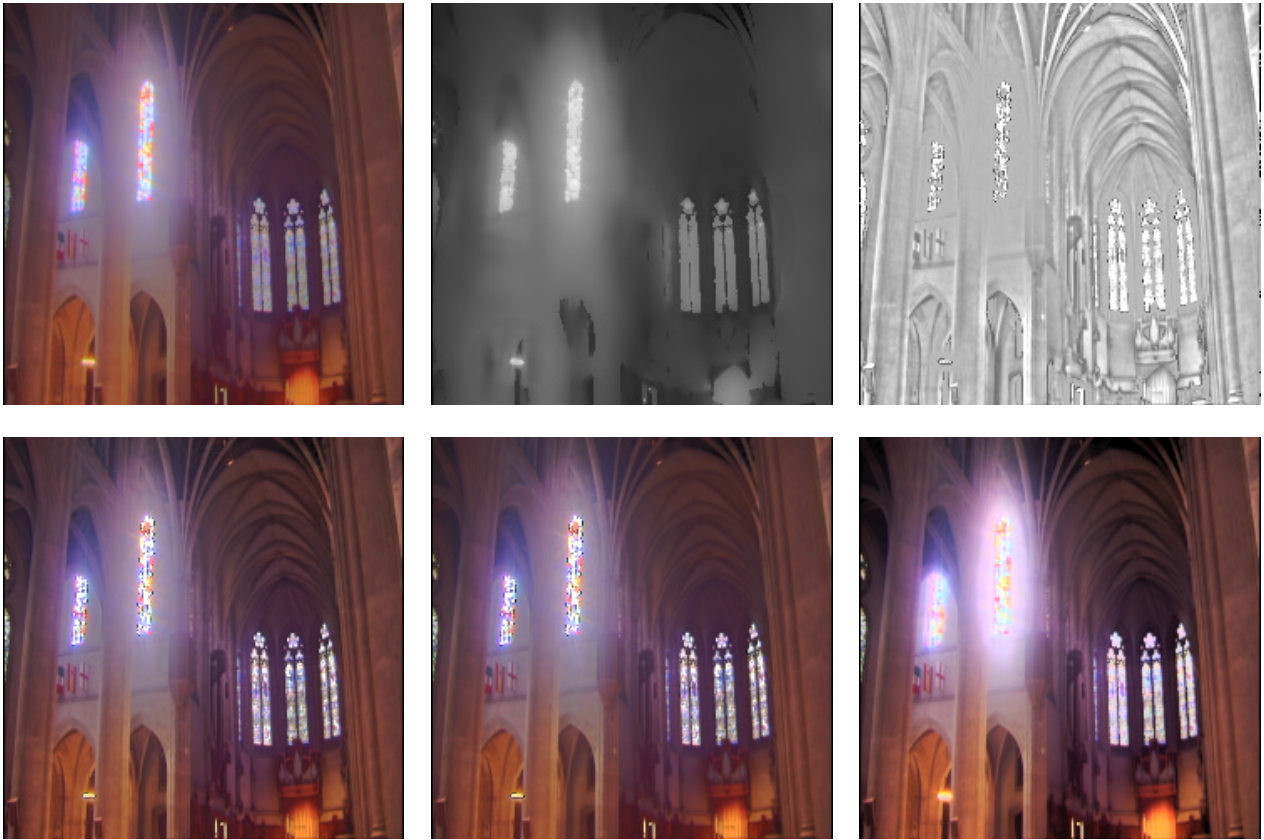
Figure 3: Operation of our algorithm. In reading order: a. application of TM(L) to pixel luminances, b. computed adaptation image after tone mapping by TM , c. details image (midlevel grey corresponds to value one), d. final result using equation 2, e. same using visible contrast definition (equations 3 and 4), f. histogram-based tone mapping 11 result.
