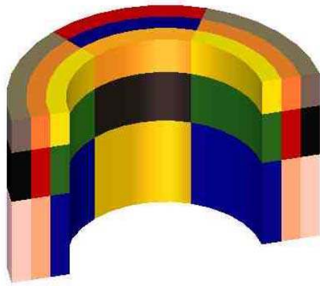
Figure 2. Cylinder liner discretization
