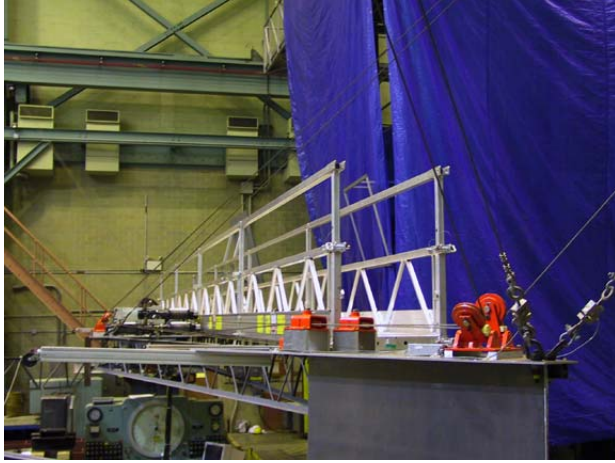
Figure 3. Full-scale Flying Carpet prototype top view shown in the ship side access configuration. The full-scale platform is near a mock ship (photo right) and in this test there was no dry dock wing wall to push against with the platform outriggers.
