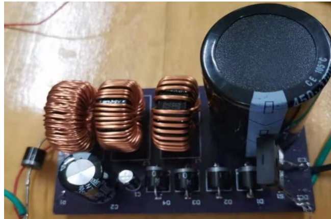
Figure 12. Hardware prototype of three-order boost converter.
