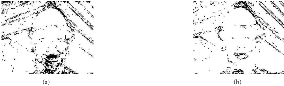
FIGURE 10: The unobservable pixels of frame 22 (a) and frame 25 (b) in the nonsynthetic “Foreman” experiment.
