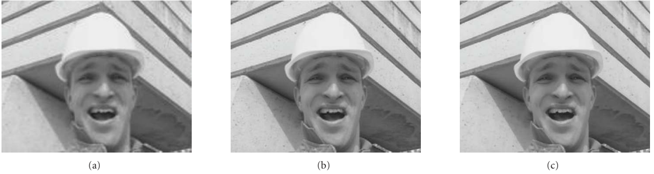
FIGURE 12: Experimental results in the nonsynthetic “motion only” case. (a) LR frame, (b) Laplacian SR result with \lambda = 0.008 and (c) TV SR result with \lambda = 0.512 .
