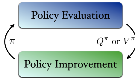
Figure 2.2: Policy evaluation/improvement loop: The convergent policy is guaranteed to be optimal, if the Q or V value functions are exact.
