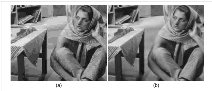
▲ 20. The “Barbara” image coded at 0.2 bits/pixel with JPEG (a) and EZW (b) using a three-level decomposition. The resulting PSNRs for the coded images are 23.3 dB (JPEG) and 24.4 dB (EZW).
