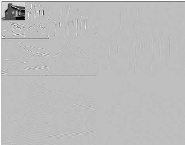
▲ 5. A three-level ( K=3 ), 2-D wavelet transform using the symmetric wavelet transform with the 9/7 Daubechies coefficients (the high-frequency bands have been enhanced to show detail).
