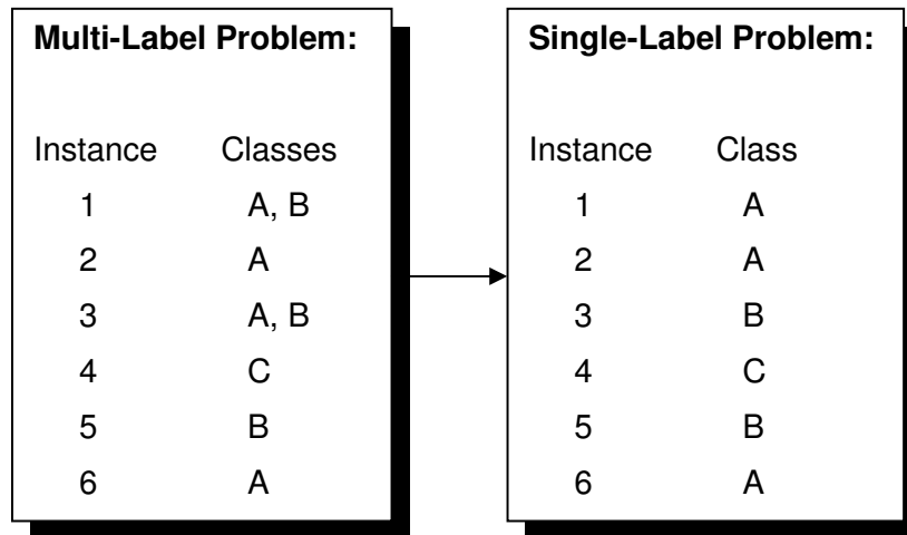
Fig. 5. Transform by label elimination of a multi-label problem into a set of single-label problems
