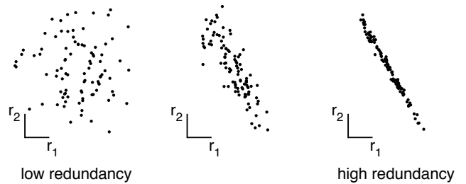
FIG. 3 A spectrum of possible redundancies in data from the two separate measurements r_1 and r_2 . The two measurements on the left are uncorrelated because one can not predict one from the other. Conversely, the two measurements on the right are highly correlated indicating highly redundant measurements.
