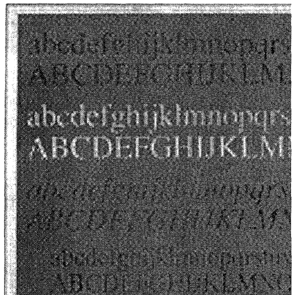
Figure 10b. A compressed version of the simulated halftone picture of Figure 10a, utilizing QMF 30:1 compression.
