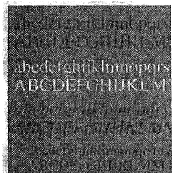
Figure 10c. A compressed version of the simulated halftone picture of Figure 10a, utilizing JPEG 30:1 compression.
