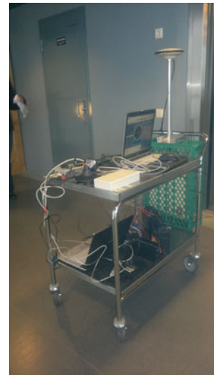
Fig. 6 Test equipment. The Nokia N8 phone acquiring the images was attached to the holder in the front of the cart
