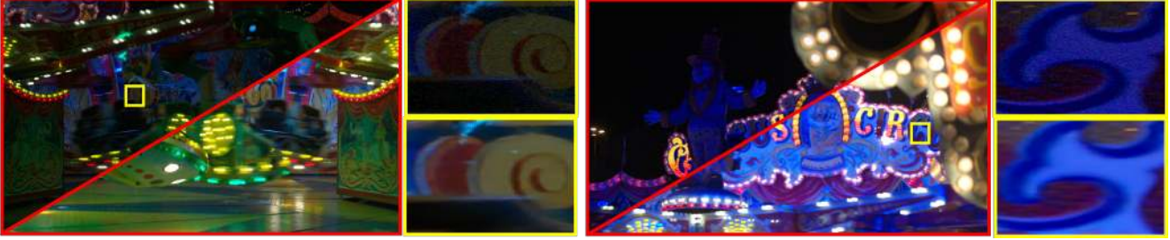
Figure 1: Single-shot LDR to HDR reconstruction obtained by the proposed two-stage deep method. The proposed network intends to map an 8-bit LDR input into a 16-bit HDR image. However, for better visualization, we normalized the reconstructed images and compared them with their inputs. In each pair, the top section illustrates the LDR input, and the bottom segment shows the corresponding HDR output.
