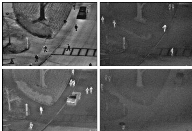
Figure 1: Thermal images showing large intensity variation.
