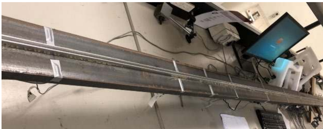
Figure 10 The installation of plastic strip to simulate bumps on the bridge
