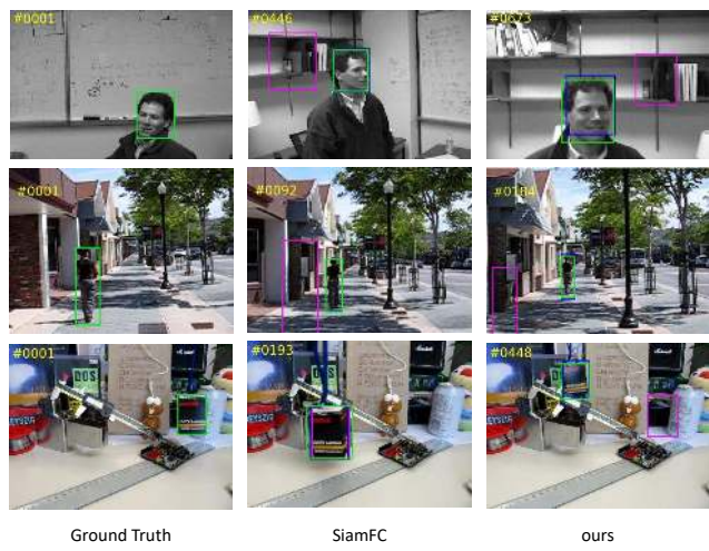
Figure 1. Comparing the tracking results of SiamFC and our tracker. Thanks to the semantic features, our tracker successfully follows the target object in case of shooting angle change or scale change, when SiamFC fails.
