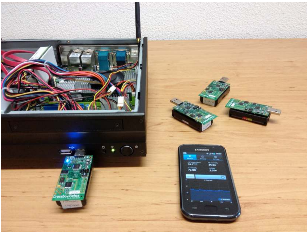
Figure 9. 6LoWPAN wireless sensor network laboratory testbed.
