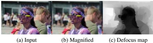
Figure 11: Defocus blur magnification. The background blurriness is amplified to direct more attention to the foreground.
