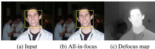
Figure 12: All-in-focus image generation. Blurry regions (yellow boxes) in the original image look clearer in the all-in-focus image.
