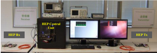
Fig. 12: Overview of the CPHY real-time implementation platform.
