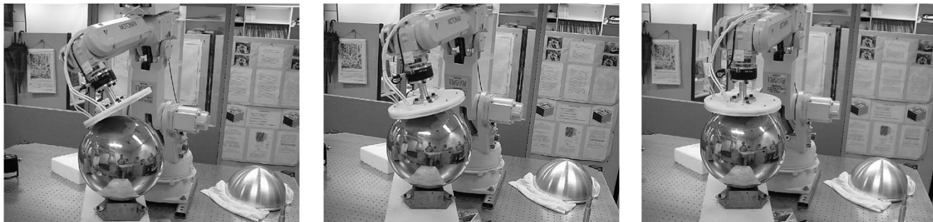
Fig. 15. Successive motion states of rolling.
