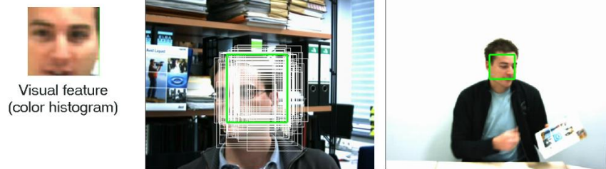
Figure 6. Color-based particle filter.
