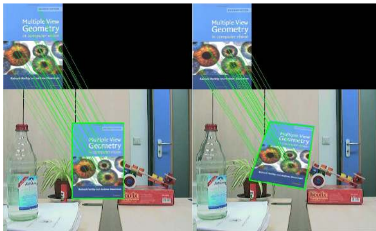
Figure 8. 3D Pose estimation with invariant keypoints - GPU-based implementation.
