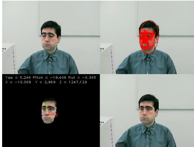
Figure 12. 3D Face tracking integrating contour and template visual modalities.
