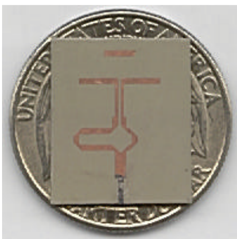
Fig. 2 Picture of an X-band prototype quasi-Yagi antenna.
