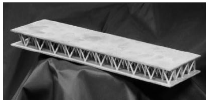
Figure 7.9 A Tetrahedral Lattice Structure Made by Rapid Prototyping Followed by Investment Casting
