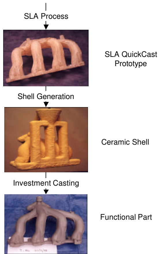
Figure 7.13 QuickCast Process to Fabricate Metal Parts and a Typical Rib Pattern
