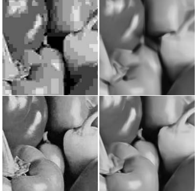
Fig. 3: Peppers at 0.14 and 0.45 bpp: JPEG (left), GMR (right)
