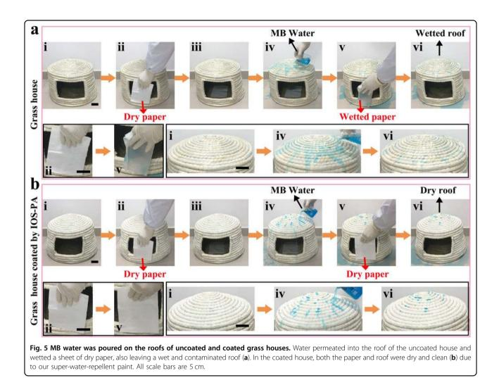
original dry paper became wetted, resulting in a wet and MB-contaminated roof. In contrast, because of the strong water repellency of IOS-PA (Fig. 5b, Supplementary Movie S11), the paper always remained in the dry state, and a waterproof roof was observed.
