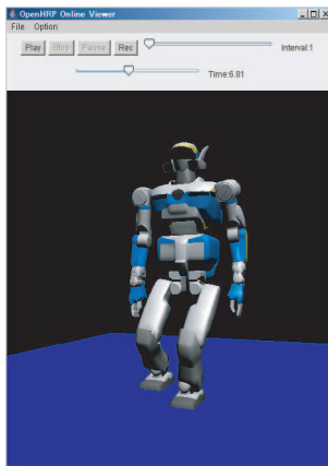
Fig. 5. HRP-2 walks on a horizontal plane with a sufficient friction
