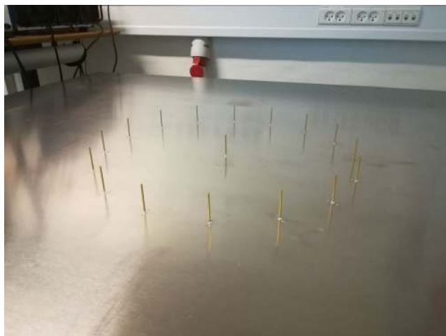
FIGURE 2. Antenna array used in the setup.
