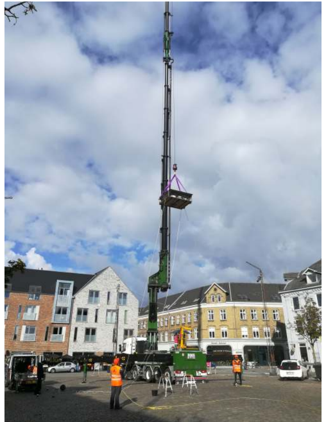
FIGURE 14. Designed testbed lifted in the air during measurement campaign focusing on a UAV A2G channel characterization.
