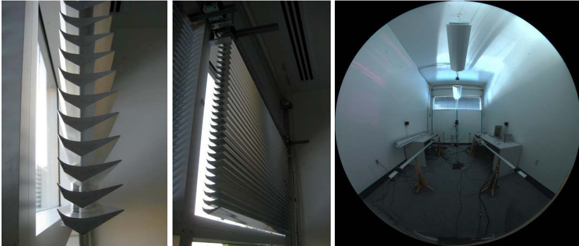
Figure 2. (left): Side view of the OLS on the inward face of the clerestory glazing. (middle): Oblique view of the OLS. (right): Photo of the test space with OLS installed (looking from the back of the space towards the window)
