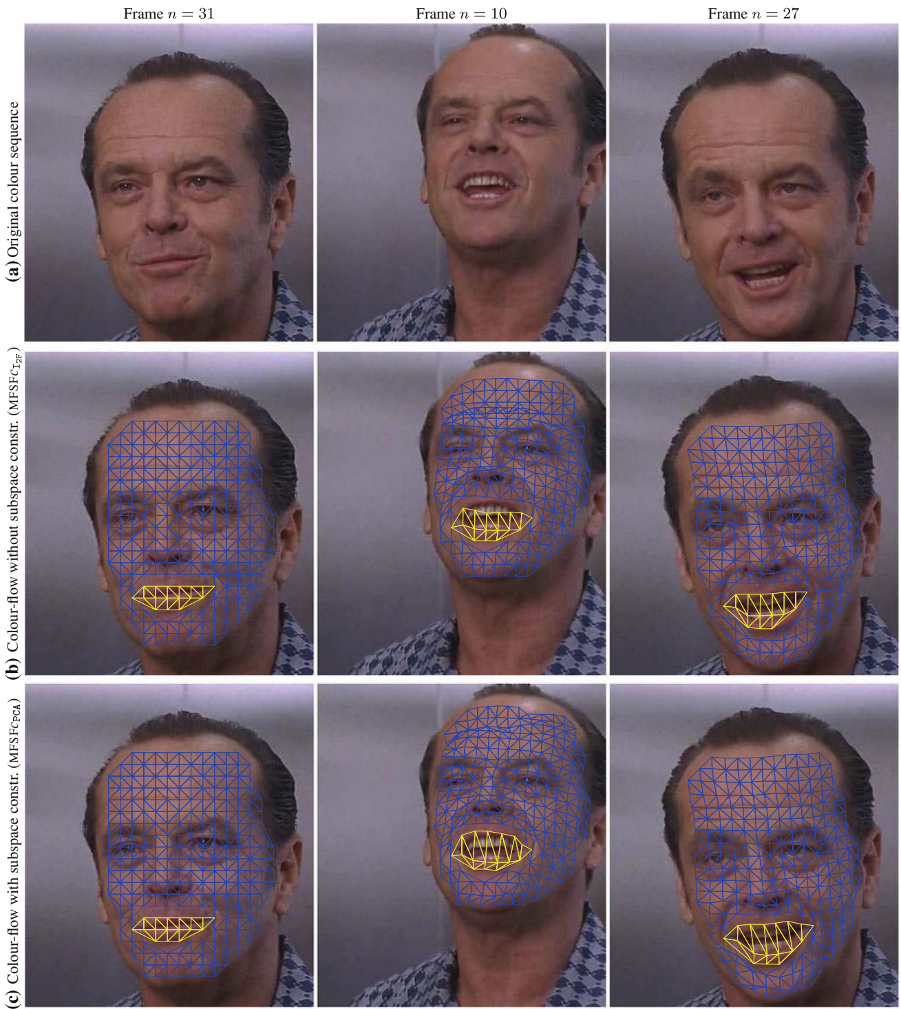
Fig. 10 Results on the colour Actor sequence: Top row (a) shows some frames of the original colour sequence. Middle (b) and bottom (c) rows compare the optical flow results obtained with two of our proposed colour algorithms: (c) with subspace constraints (MFSFc PCA ) and (b)
