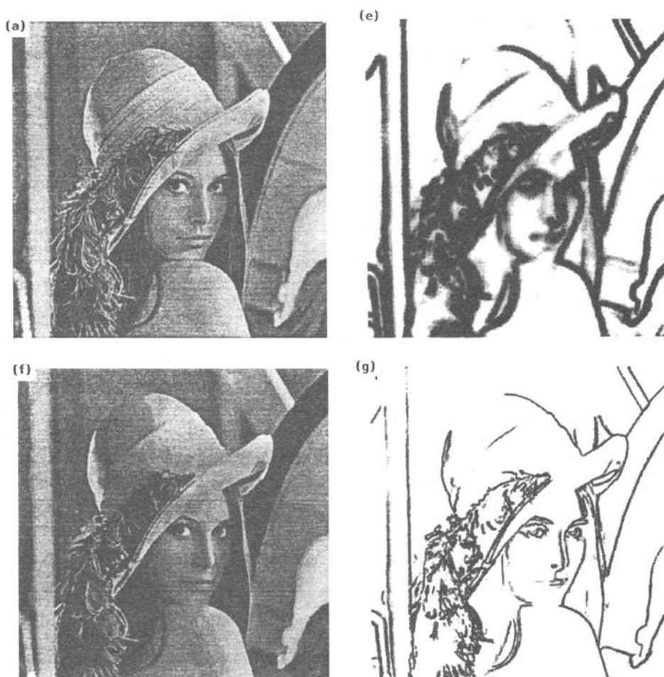
Figure 6. (a) Lenna image 512 \times 512 . Prescaling \Phi(v) (b), final f (c), and final \Phi(v) (d), with initial parameters \beta = 0.0025 , \alpha = 0.05 , c(0) = 2.0 and final parameters \beta = 0.025 , c = 0.2 . Prescaling \Phi(v) (e), final f (f), and final \Phi(v) (g), with initial parameters \beta = 0.004 , \alpha = 0.03 , c(0) = 2.0 and final parameter \beta = 0.04 , c = 0.2 .
