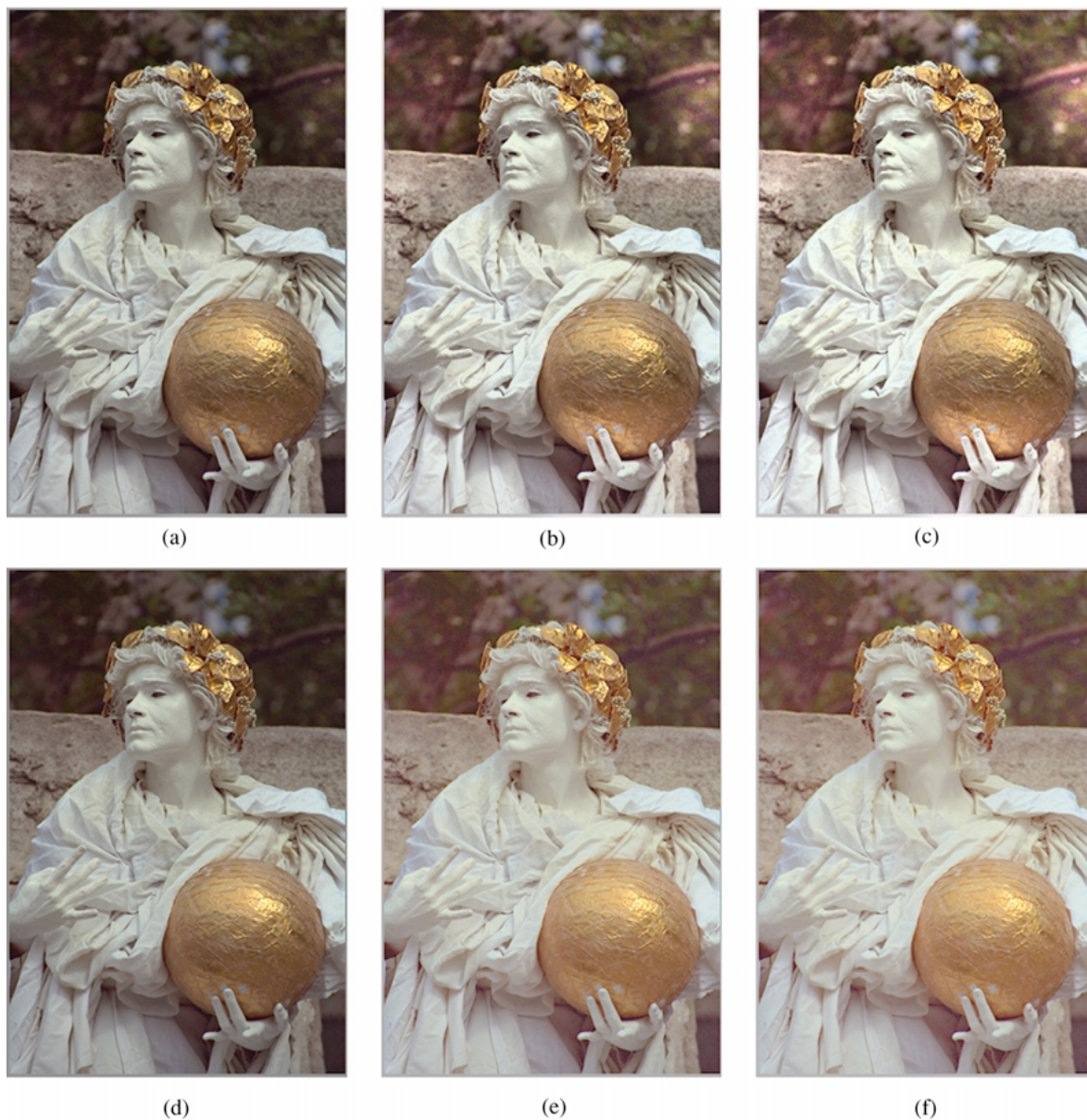
Figure 9. The influence of \gamma (illumination return) compared to standard Gamma correction; The proposed algorithm with \gamma = 2 in (a), \gamma = 6 in (b), and \gamma = 24 in (c). Standard Gamma-correction with \gamma values tuned to fit corresponding output of the proposed algorithm: \gamma = 1.4 in (d), \gamma = 2.1 in (e), and \gamma = 2.4 in (f).
