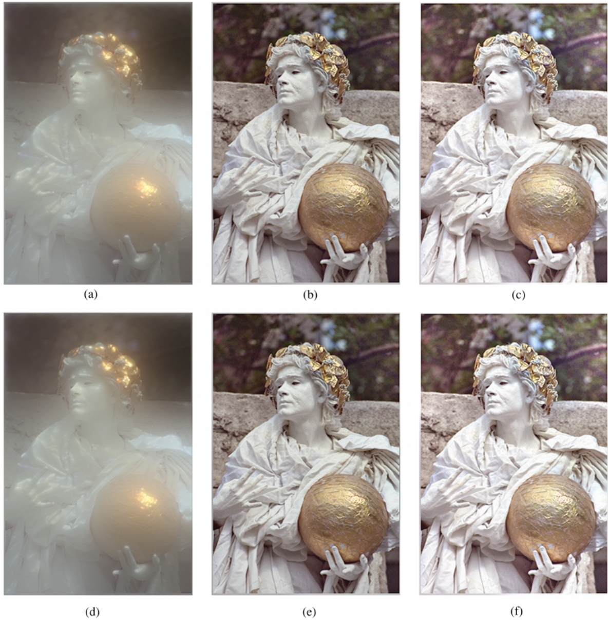
Figure 5. Invariance to gamma-correction: (i) Top row—direct application of the Retinex procedure, with illumination in (a) output with \gamma = 3 illumination return in (b), and output with \gamma = \infty illumination return in (c); (ii) Bottom row—inverse gamma correction before and gamma correction after the Retinex procedure using \gamma = 2.2 , with illumination in (d), output with \gamma = 3 illumination return in (e), and output with \gamma = \infty illumination return in (f).
