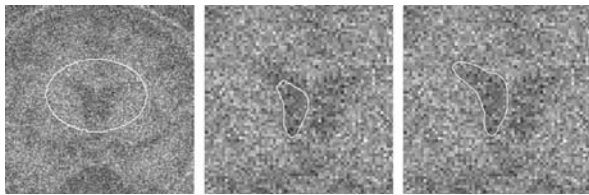
Figure 21. Evolution of the active contour (in solid line) with a shape prior (in dotted line) in the presence of an important quantity of noise.
