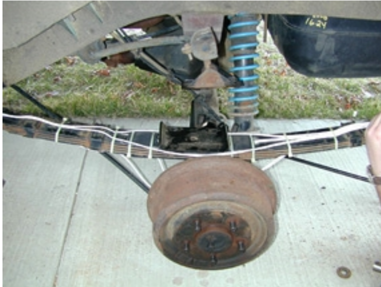
Figure 3. Strain gauge testing of an SUV leaf spring fitted with the Articulating Lift Block.
