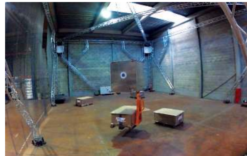
Fig. 2. LIRMM/TECNALIA CoGiRO suspended CDPR prototype.
