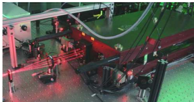
FIG. 4. (Color online) Photograph of the JILA-MONSTR highlighting the input beam on the right-hand side of the picture and four output beams focused to a single location.
