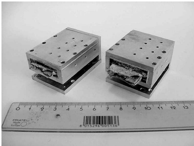
Fig. 11. Photograph of the two structures. Left: indirect heat removal; right: direct heat removal.
