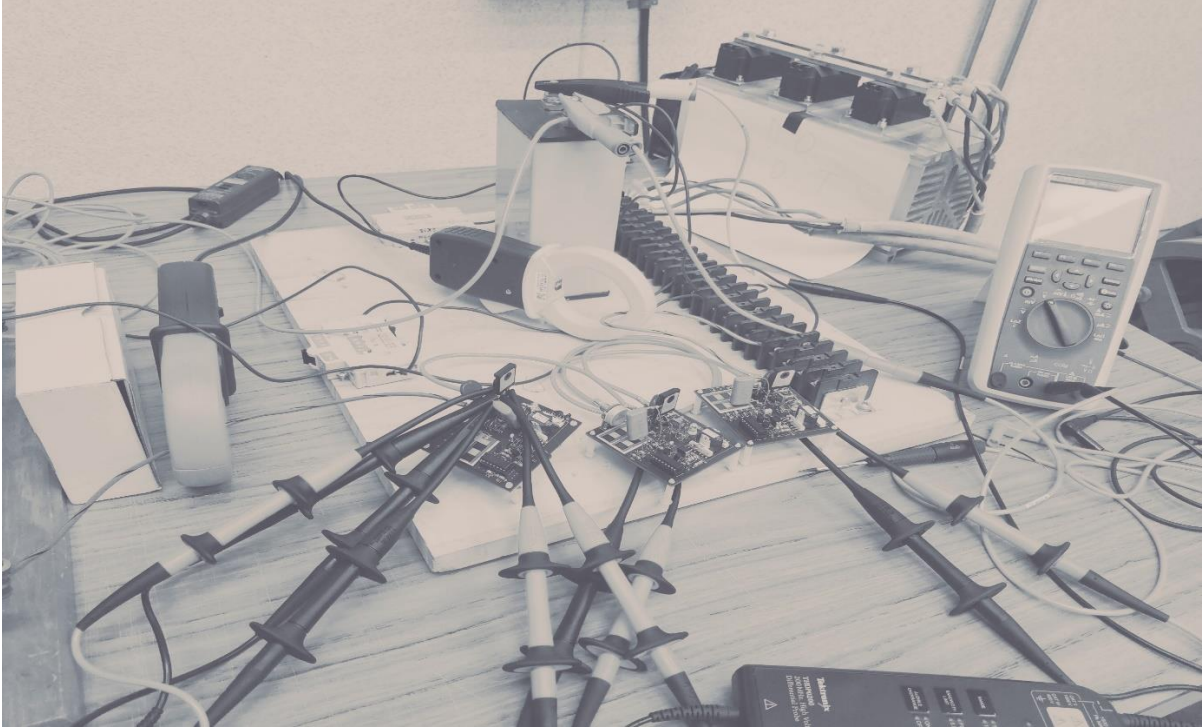
Figure 7-19 – Cascaded JFET experimental set-up
