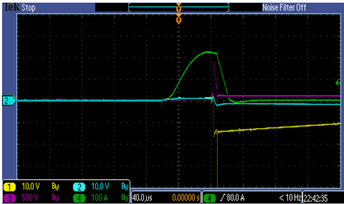
Figure 7-20 – Cascaded SSCB Scope 1 Plot in the Lab. Ch 1(VGS1) - 10V/Div, Ch 2(VGS2) – 10V/Div, Ch 3(VDS1) – 500V/Div and Ch 4(IDS) 100A/Div.
