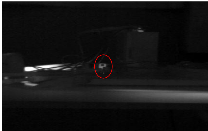
Figure 7-8 – Single JFET Thermal Image
