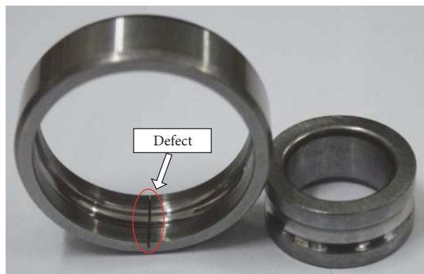
(b) Localized defect on the outer raceway
