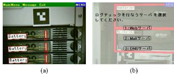
Figure 14: Red boxes are displayed on the screen to highlight the LED indicators on the UPS (Figure (a)). The user can see both the instruction and the real environment simultaneously.
