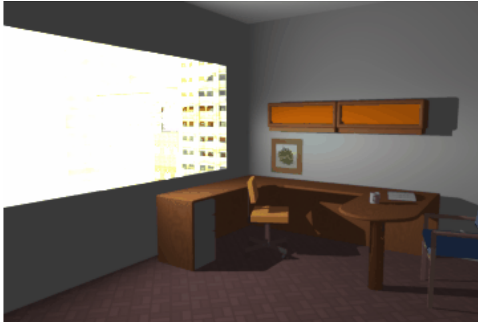
Figure 2. A linear mapping of the luminances in Figure 1 that over-exposes the view through the window.
