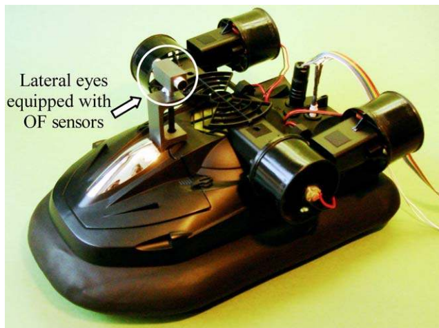
Fig. 1 Sighted fully actuated hovercraft developed for testing the LORA III autopilot. Four ducted fans (GWS EDF-50, PMW-controlled DC motor CN12-RLC) drive the robot in the plane. The hovercraft is a retrofitted version of a miniature RC hovercraft (Taiyo Toy Ltd., Typhoon T-3: 0.36 \times 0.21 \times 0.14 m). The robot is equipped with two lateral eyes looking at an angle of \pm 90^\circ to the side, each of them driving a single OF sensor comprised of a pair of PIN photodiode. An additional brushless DC motor actuates the airbag turbine
